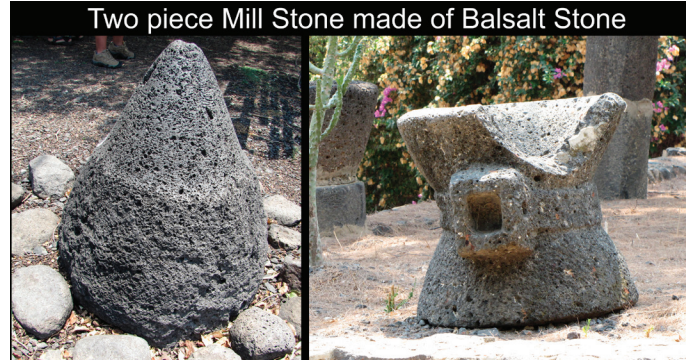
1. The bottom stone formed like a cone with a circular trough around the bottom of the cone to catch the grain after it had been ground. 2. The top stone shaped like a cylinder with an open shaft through the middle to pour the grain. This was placed on top of the cone shaped stone and rotated with a wooden beam or handle.
