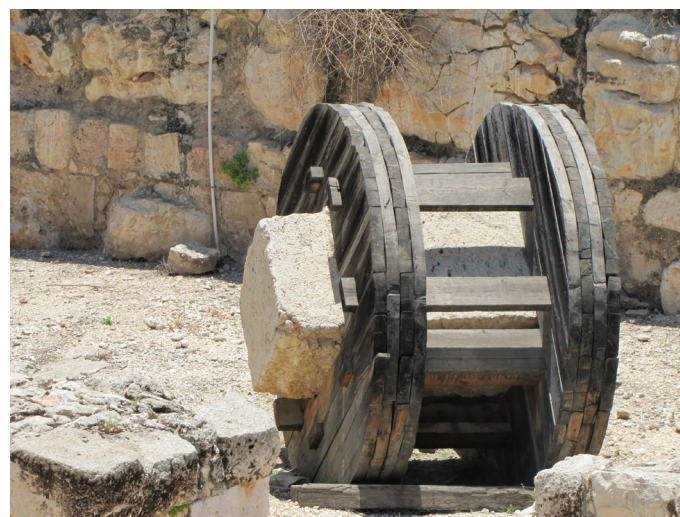
Ashlars were placed in rollers like this to be moved to location. This was one of several ways the stones were moved. Stones were also pulled by teams of oxen on rollers.
